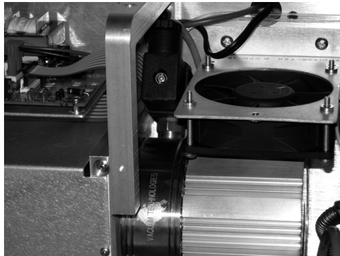
Figure 1-7b. Detailed view of the TP vent valve configuration
