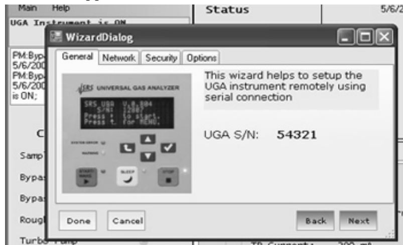
Fig. 2-7. Screenshot of the 'Wizard' dialog box in the Main menu of UGA control software.
