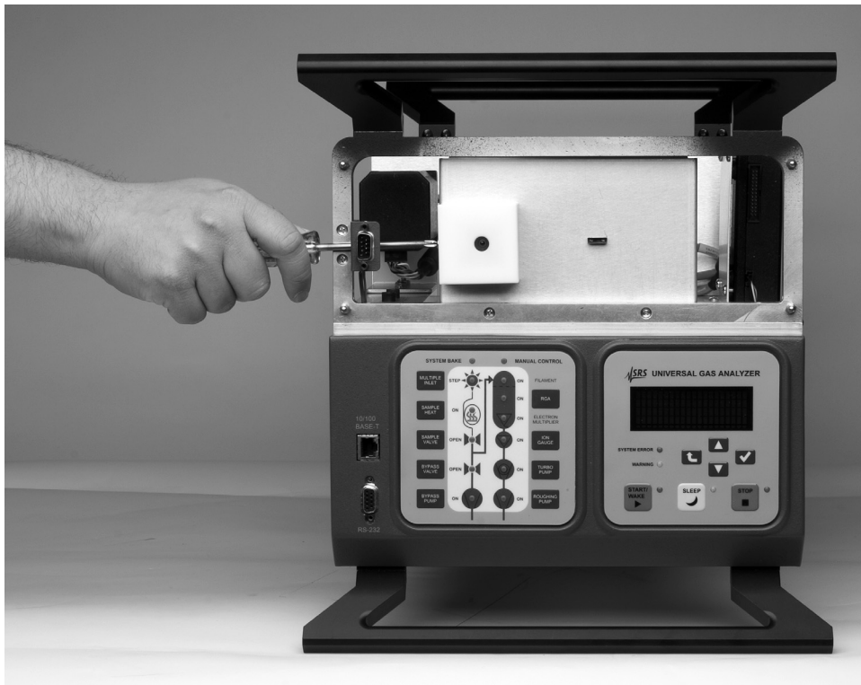
Figure 1-11. Ultra-Torr insulator releasing for O100HC capillary change or connection
